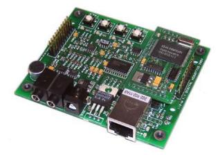
The **OEM Module** is designed for system integrators and OEMs who wish to add two-way audio communications to their systems. Using Digital Acoustics' patent-pending technology, intercoms are easy to connect and offer both audio transport and multiple GPIO ports. "Personality modules" allow connection to various I/O devices.
