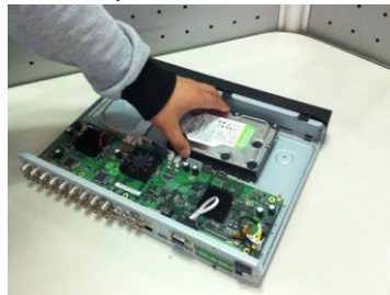
3. Place the HDD in accordance with the four holes in the bottom.
