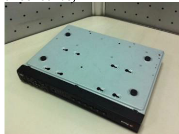
4. Turn the device upside down and then turn the screws in firmly.
