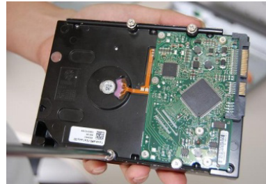
2. Fix four screws in the HDD (Turn just three rounds).
