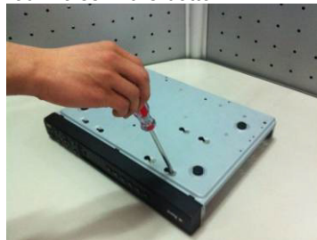
5. Fix the HDD firmly. .
