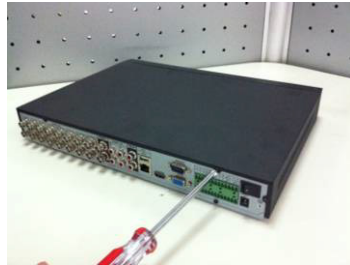
1. Loosen the screws of the upper cover and side panel
