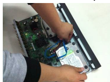
6. Connect the HDD cable and power cable.
