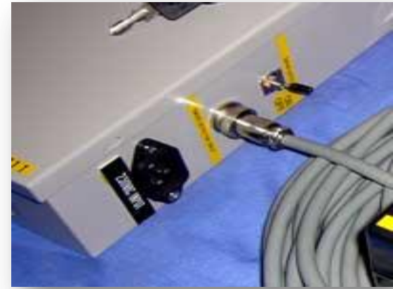
Smoke Detector Control Power input and Connector and ON/OFF switch
