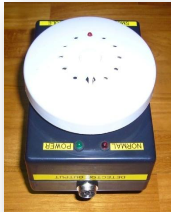
Smoke Detector Module signal input & system LED indicator
