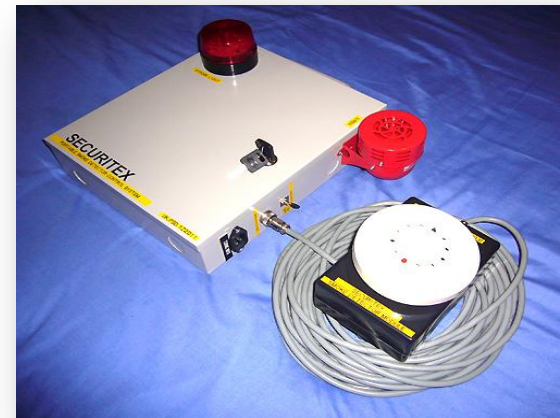
Smoke Detector Control System c/w complete Individual module
