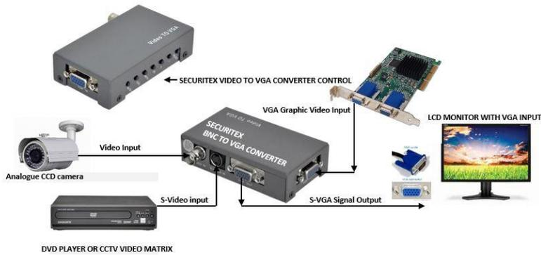
The above diagram shows how simple it is to use this converter to connect an analogue CCTV camera to a VGA monitor input. The CCTV camera is wired to the BNC to VGA converter using RG59 coax cable. The VGA output of the converter is attached to the input of the monitor using a standard VGA cable.
