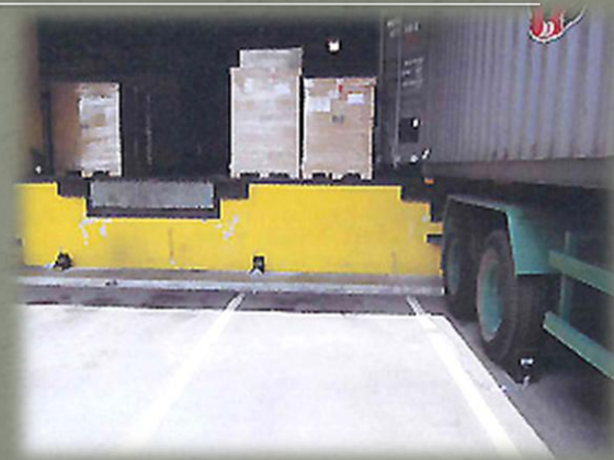
SECURITEX WHEEL CHOCK TO CHOCK CONTAINER WHEELS CHOCK IS CHAIN TO THE LOADING & UNLOADING BAY
