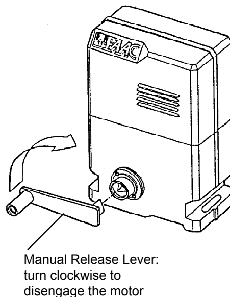
Figure 3. The Manual Release Lever on the 820 and 860 Operators
