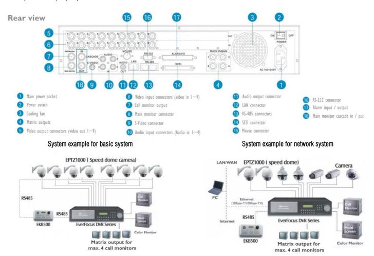
EEPbus remote control with speed dome star wiring
