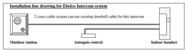
Specifications: Power source: DC 6V (LR 6-AA). Power supply: Batteries only, 4 pieces X 1.5 V (6V). Consumption: In use 30mA, Chime signal 150mA. Signal sound: Electronic chime call sound. Wiring: 2 wires installation. Communication range: Distance 300 metres-diameter 0.65mm cable gauge.
