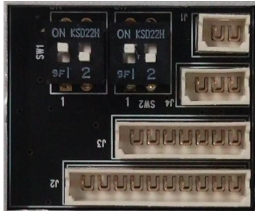
(Figure: The Position of SW1 and SW2 to generate Weigand Output Format)
