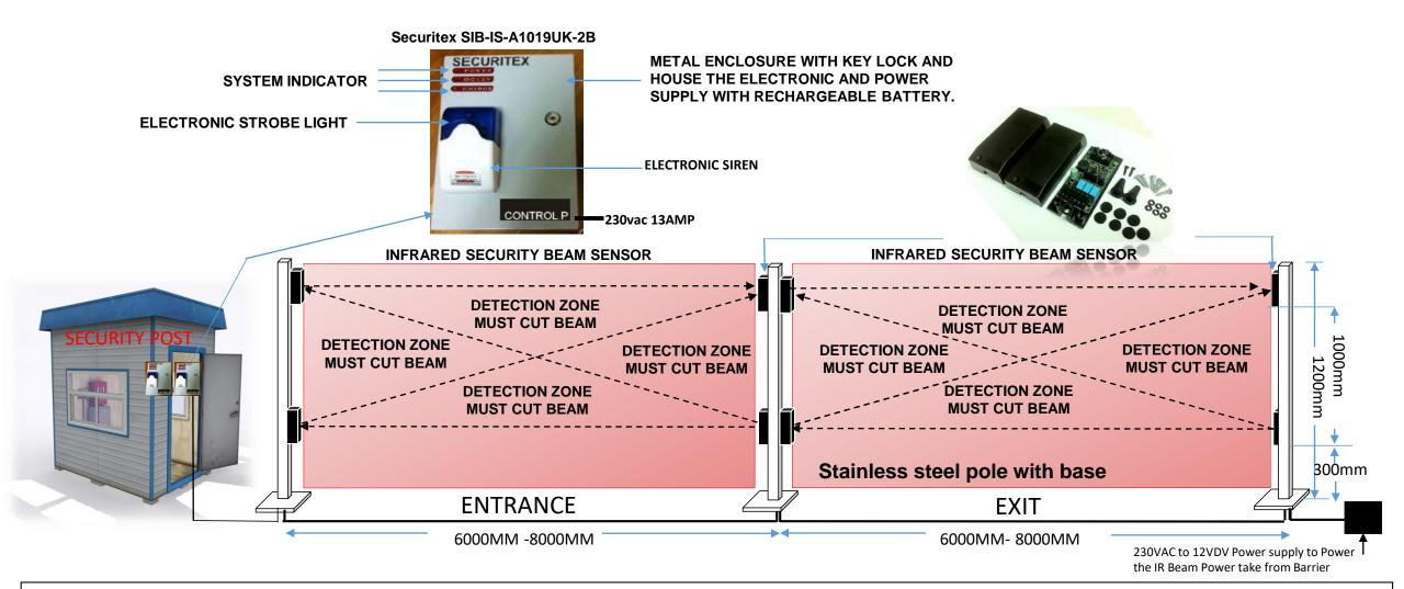
SYSTEM NAME: SECURITEX SIB-IS-A1019UK-2B APPLICATION: SECURITEX INFRARED BEAM INTRUSION & ALERT SYSTEMS
