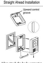
After attach the body supporter with 2 screws. put the Door Camera into the grooves of body supporter, and then fix it with a screw.
