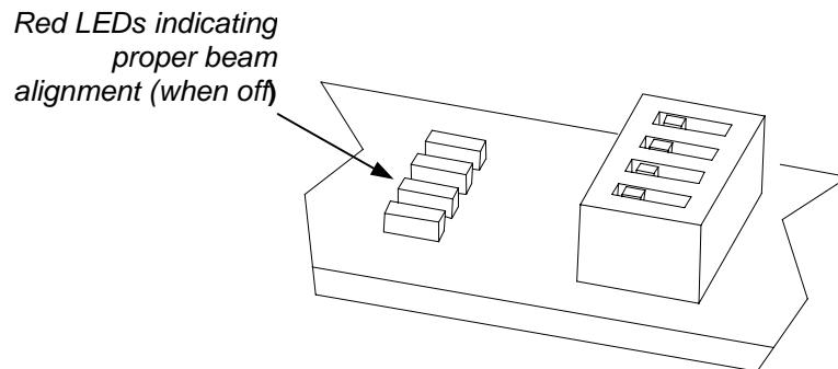
10. Check for easy beam break off by cutting off the TX Master to RX Slave beam and verifying that both the Master and Slave red LEDs come on, whereas cutting off of the TX Slave to RX Master beam should cause only the red LED on the Master card to come on.
