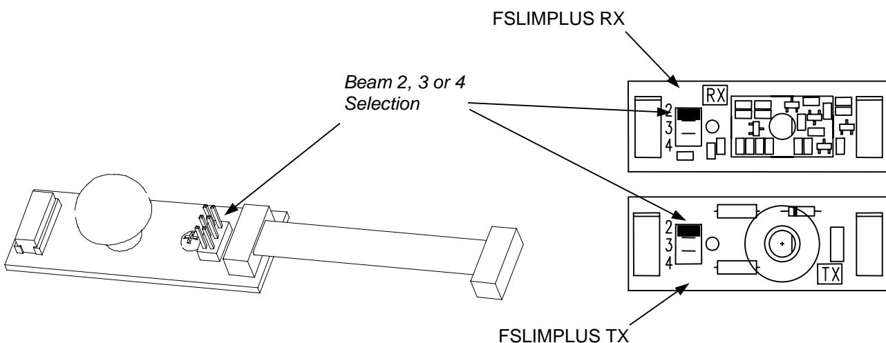
8. Set "BEAMS" DIP SWITCHES in the MASTER and SLAVE cards, of beams being used, to **OFF**.
