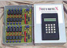
Telephone elevator controller
