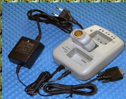
TouchChecker Data Transmitter with Power adapter & Data cable
