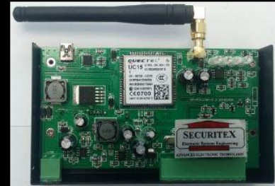
3G Network Control Interface
