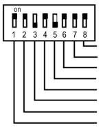
Not used Wiegand Data 0 Bias Wiegand Data 1 Bias Single/Dual LED CNTL KeyPad Green LED Control Beeper Control Hardware Identity Default Setting
