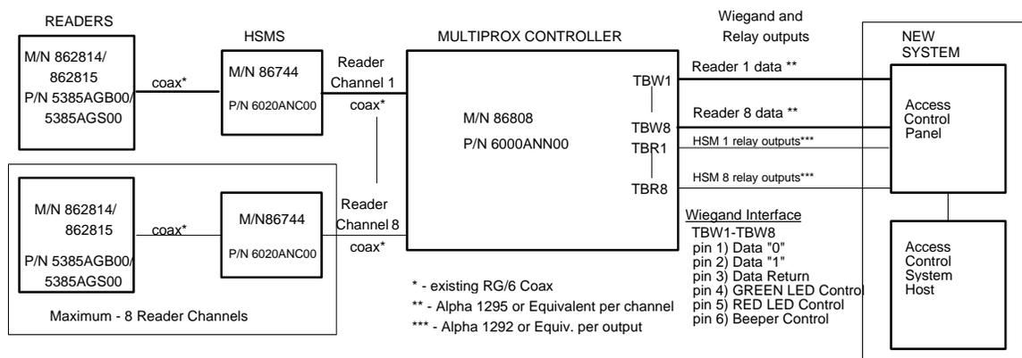
Note - HSMs are only required when input (REX/Door Sense/ Aux. inputs) wiring is local to the reader door.
